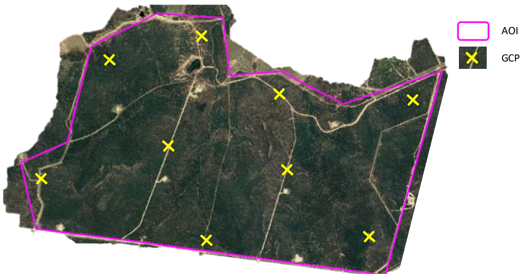
Figure 3. Typical layout of GCPs across a larger, more complex AOI
