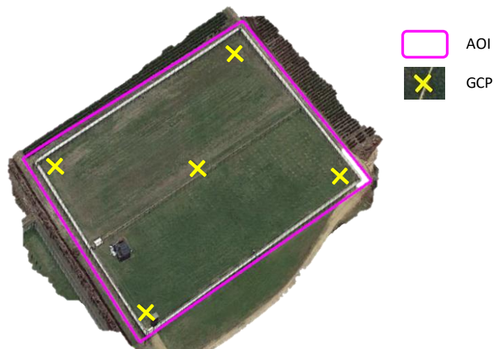
Figure 2. Standard GCP layout for a simple aerial survey of a small area.
