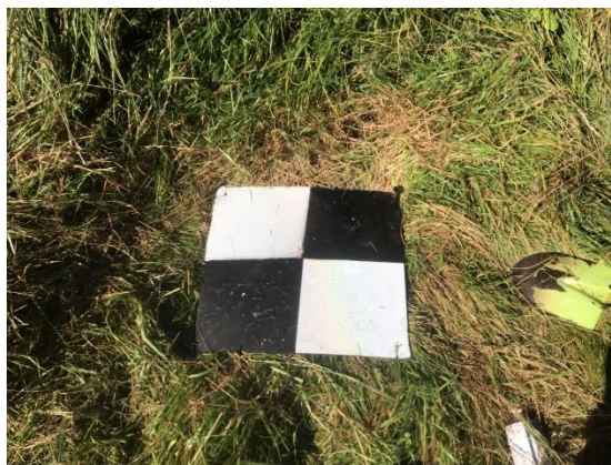
Figure 4. Retroreflective lidar target in use in the field.
